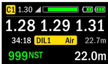
During the dive the oxygen controller controls the oxygen partial pressure in the breathing loop by averaging the nearest two cell output readings, i.e. if you have one cell reading 1.28, another 1.29 and the other 1.31, the cell displaying 1.31 will be ignored and the ppO<sub>2</sub> assumed to be 1.285. As it is below the setpoint, the solenoid will open for a fraction of a second.
