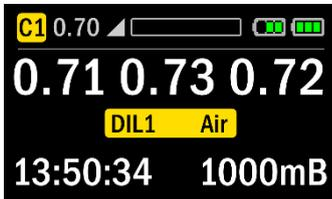
When first breathing on the rebreather, a rapid drop in ppO<sub>2</sub> will be seen. Obviously the drop in ppO<sub>2</sub> occurs because the exhaled breath contains only about 17% oxygen and you are forcing the oxygen pressure down very quickly. If you stop breathing into the loop, just take it out of your mouth, you should then expect to see the ppO<sub>2</sub> rise rapidly back towards the setpoint.
