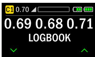
Press the centre button to enter Log Book. Scroll through dives using the arrows to see the dive Number. on the top line, the date (dd/mm/yy) and dive duration (mins/secs), on the 2<sup>nd</sup> line, time of entry(hrs/mins/secs) and maximum depth (metres or feet) on the third line.
