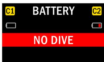
On switch on, if both batteries are displaying one square or less - BATTERY – NO DIVE is displayed, the oxygen controller will not continue into dive mode and the dive cannot commence.
