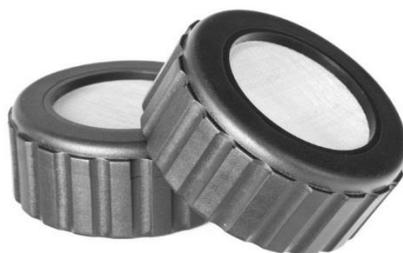
The Cell validator is supplied with “thread protection caps”, which when removed from the cell validator can be attached to the rear side of each T-piece. The caps have stainless steel mesh panels to allow the inner bags to “breathe” but also prevent insects from entering.
