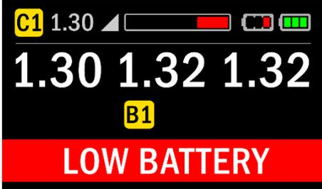
Whenever a warning is active on the display, the top bar information will be shown along with the warning but the compass details will still be shown as the warning alternates with the depth, time and decompression information.
