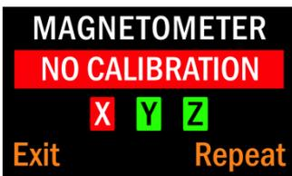
If the handset is not rotated sufficiently enough during either calibration process to give an accurate calibration, a 'NO CALIBRATION' screen will be displayed. This will indicate which plane did not receive enough rotations with a red box. In the first example the X plane caused the failed calibration and in the second example, it was the Y and Z. Simply select 'Repeat' and attempt to rotate the handset again or select 'Exit' to continue without calibrating the compass.
