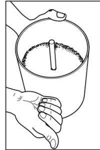
Fill to approximately half way and tap gently on the sides to level the granules
