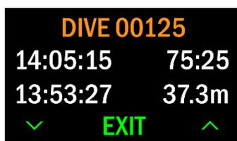
The dive No. is incremented by one every time the rebreather descends below 1.2m providing the surface interval is greater than 5 mins. If the surface interval is less than 5 mins it is counted as an extension of the previous dive. Press the centre button to exit Dive Log. The dive end is logged when the depth display is at approx. 0.9m (3ft) or shallower.
