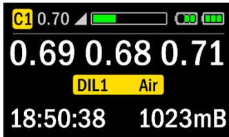
**NOTE:** When in demo mode the Scrubber monitor scrolls to indicate it is in dive mode. The left button does not call up the Slave display (whilst in demo mode). The setpoint is automatically set at 0.70 bar and the Low Oxygen warning is set at 0.16 bar, which eliminates nuisance beeps during demo mode use.
