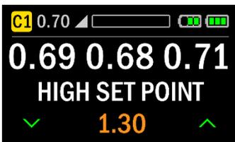
The default high setpoint is 1.30 bar but is adjustable from 0.9 to 1.5. It always defaults back to 1.3 when the electronics are turned off.
