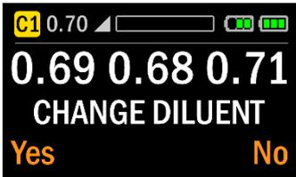
CHANGE DILUENT is a closed circuit option and is displayed if a “No” response is given to “OPEN CIRCUIT”.
