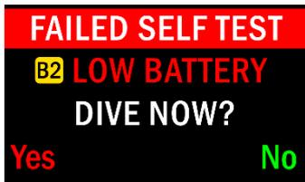
This warning screen shows battery B2 as low or missing. If YES is selected to DIVE NOW the Battery Test Screen will appear as before. A further warning screen will appear after the solenoid “load” test has been conducted.
