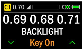
If Key On is selected, the backlight is normally off but comes on when a button is pressed. The left button operates the backlight for 5 seconds, the centre or right button operates the backlight for 15 seconds.
