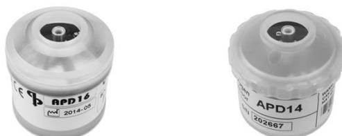
Three galvanic oxygen sensors are fitted to each rebreather. Two types are currently used, APD14 and APD16, each from a different manufacturer. Both feature the SMB co-axial connector, hydrophobic membranes and other common characteristics to allow use in the high humidity and temperatures experienced inside the breathing circuit.
