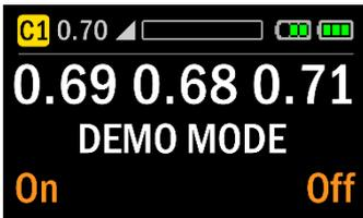
On pressing the centre button the option to turn the Demo Mode on or off is given. Select On and then arrow down to "Exit Menu" or just wait for 15 seconds.
