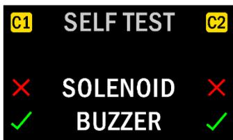
If the solenoid is not seen by both controllers then the electronics will not go into Dive mode and the connection or solenoid must be fixed prior to use.
