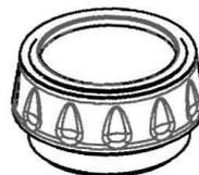
Do vent the lid after each dive for 3mins to ensure the sensor protector does not become saturated between dives.
