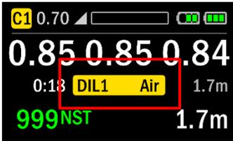
The selected diluent is shown in the centre of the display: Diluent 1, which is Air. On the deco versions there are up to 10 diluents, all of which are user adjustable and stay in memory once set.
