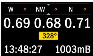
Press and hold the right button and switch the compass on. With the compass activated, press the left and right buttons simultaneously to show the menu options.
