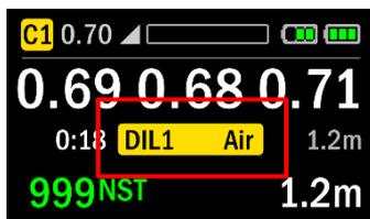
The diluent No. and description is shown on the third line. The diluent can be changed at any time, through the menu, to any of the other five stored diluents. At any time the diver may change the gas percentages of a particular diluent and this new gas will be stored for subsequent dives.
