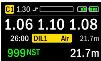
High setpoint selected (1.30bar). Oxygen is now injecting to bring the ppO<sub>2</sub> up to 1.30. The
