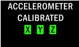
After 15 seconds, the accelerometer will also calibrate successfully as long as all three planes showed green bars.
