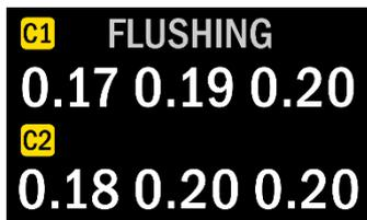
A lot of information can be gleaned during the flushing process with regard to the health of the oxygen cells. It is easy to compare the cell reaction speeds to oxygen and it is possible to see whether the cells have reached close to their full potential. The flushing process lasts until the cell outputs are stable.
