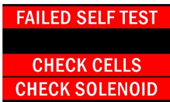
The electronics will not go into Dive mode and the connections must be fixed prior to use.
