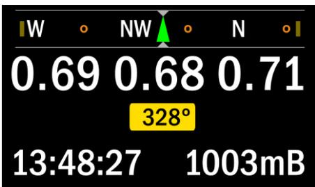
The heading is shown as a green arrow on the inner band. As you change direction the marked heading will scroll with the cardinal points on the inner band, giving an indication of which way to turn to get back to your original heading.
