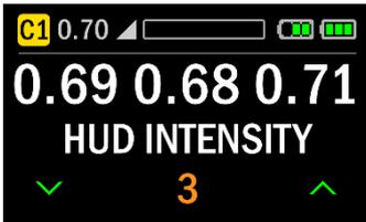
The intensity of the head up displays' LEDs may be altered to suit the ambient light. A night dive may require a lower intensity. Adjustment range is 1 to 10.
