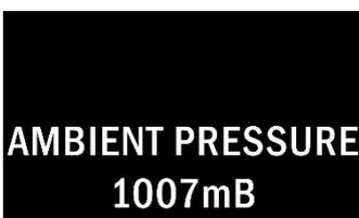
The ambient pressure is measured and displayed for a short period.
