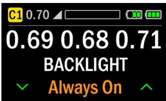
Press the right button to get to "Always On" - a useful feature on a deep dive or in cave but remember the battery drain will be much faster and MUST be monitored closely.
