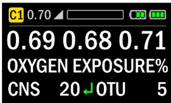
CNS and OTU are tracked in real time and displayed in the underwater menu. When 100% is exceeded appropriate warnings are displayed, these can be suppressed for 20 mins at a time.
