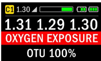
A daily OTU limit of 300 is used for the 100% indicator. A warning is raised at 100% of 300, see 3.5.7
